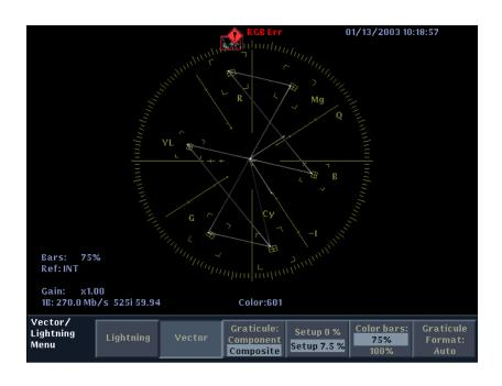
Figure 2-34: Vector display with composite graticule selected
