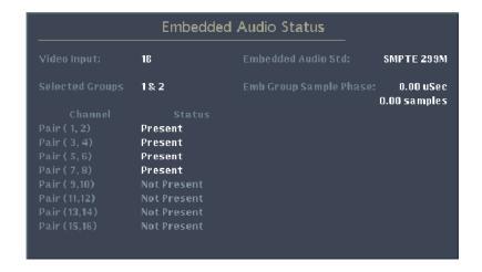
Figure 2-51: Embedded Audio Status display with HD signal
