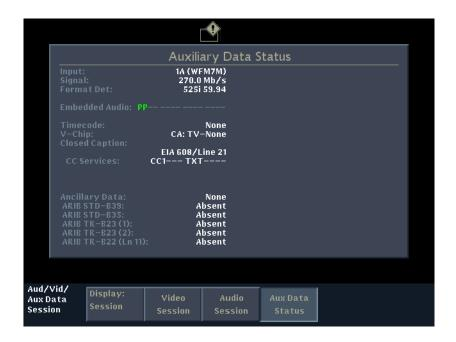
Figure 2-41: Auxiliary Data Status display
